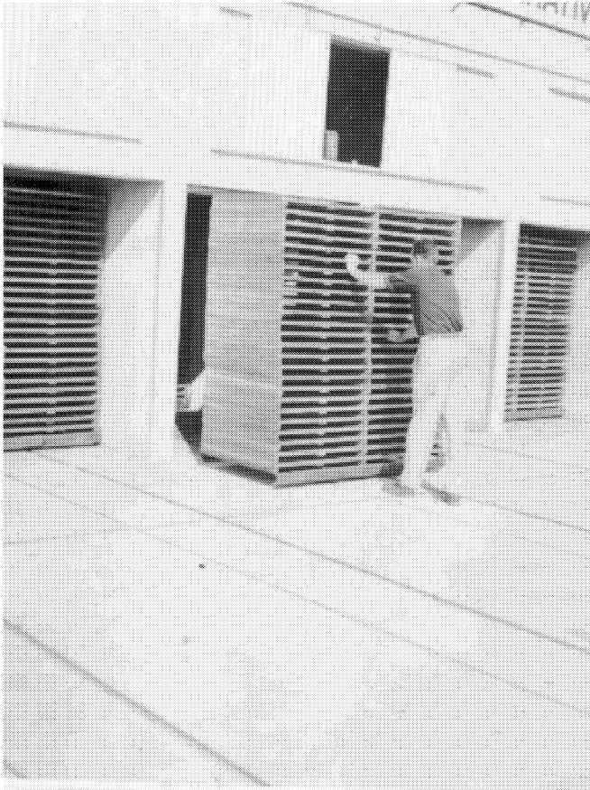
Figure 10.20. Cars of trays being moved into a tunnel drier. Note the tracks used to guide the cars. (Courtesy of California Prune and Apricot Growers Association.)
