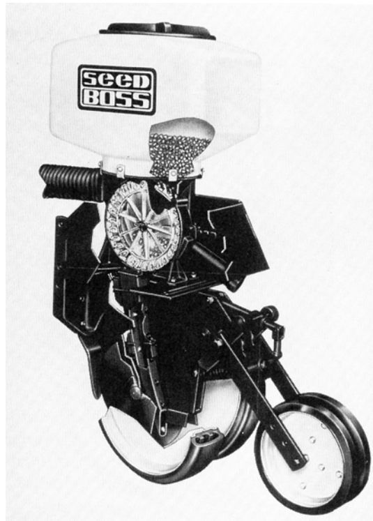
Figure 9.13 – Pressure-disk metering of seeds (courtesy of White Farm Equipment Co.).
