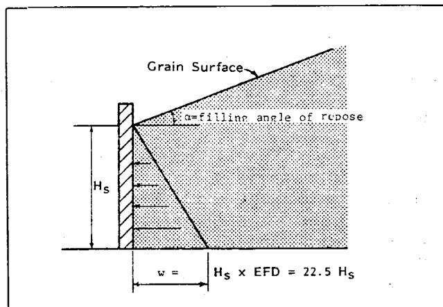
**Fig 410-3. Grain surface at the filling angle of repose.**
