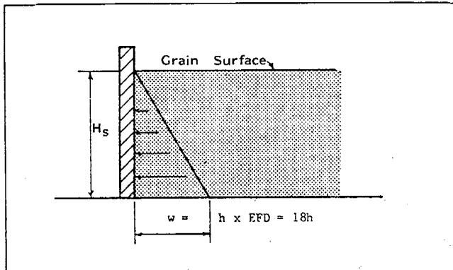
**Fig 410-2. Load on a wall from a flat grain surface.**
