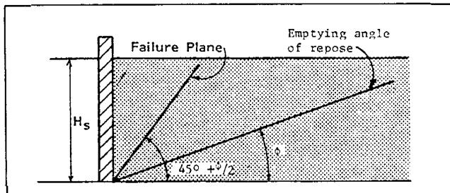
**Fig 410-1. Failure plane and emptying angle of repose in grain.**
