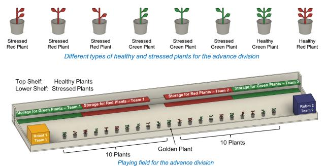
The board for the advanced division has the storage area arranged in two shelves. The advanced robot needs to place the healthy plants on the top shelf and the stressed plants on the lower shelf. No black tape will be placed on the board for the advanced robots.
