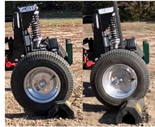
Figure 37: Comparison at 6.5mph of Suspension (left) and No Suspension (Right) with Radial Tires at 8 psi.
