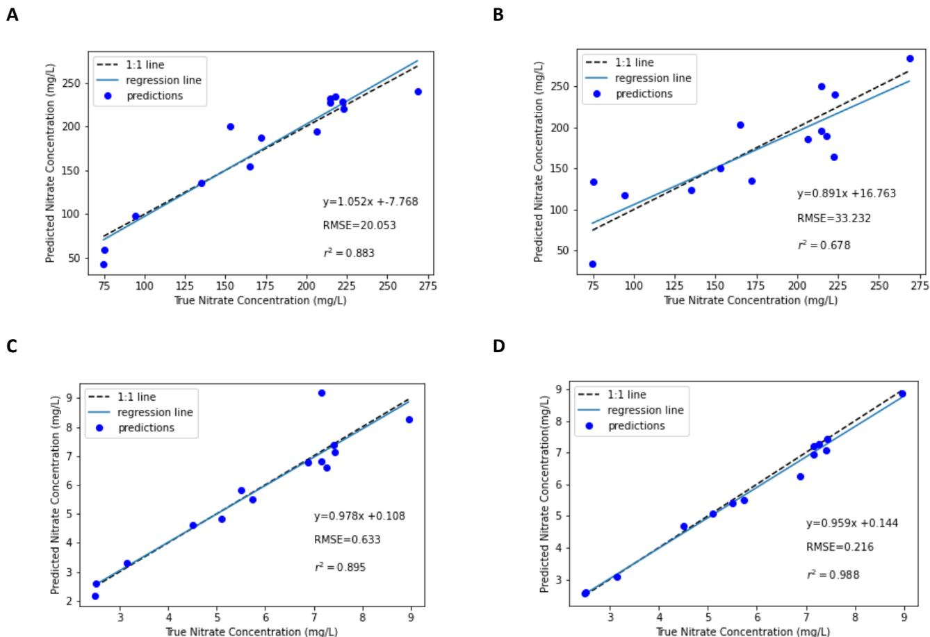
Figure 5: PLS results for predicting nitrate concentrations based on the absorbance of (A) undiluted samples produced by the NanoDrop, (B) undiluted samples produced by the GatorSpec, (C) diluted samples produced by the NanoDrop, and (D) diluted samples produced by the GatorSpec.
