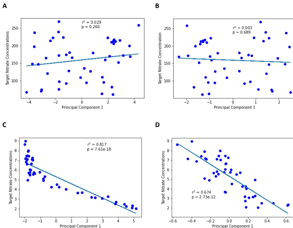
Figure 4: Target nitrate concentrations versus the first principal components produced by the UV-Vis analysis of (A) undiluted samples by the NanoDrop, (B) undiluted samples by the GatorSpec, (C) diluted samples by the NanoDrop, and (D) diluted samples by the GatorSpec.
