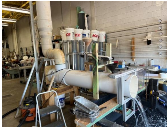
Figure 9. Hydrograph generator and slot in action
