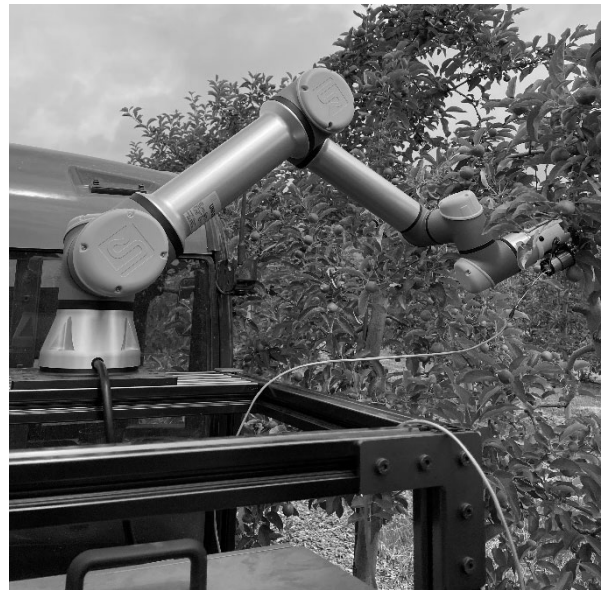
213 214 Figure 5. Field tests of the green fruit thinning end-effector, left) handheld type, and right) attached to a six DoF 215 robotic manipulator
