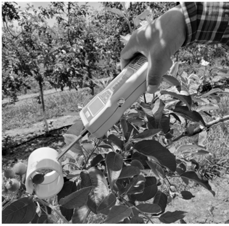
100 Figure 1. Test setup for green fruit removal force measurement, a) pulling force measurement, b) stem-cutting force 101 measurement (1: stem-holding mount; 2) stem-cutting blade; 3) digital force gauge; 4) force-transfer rod)
