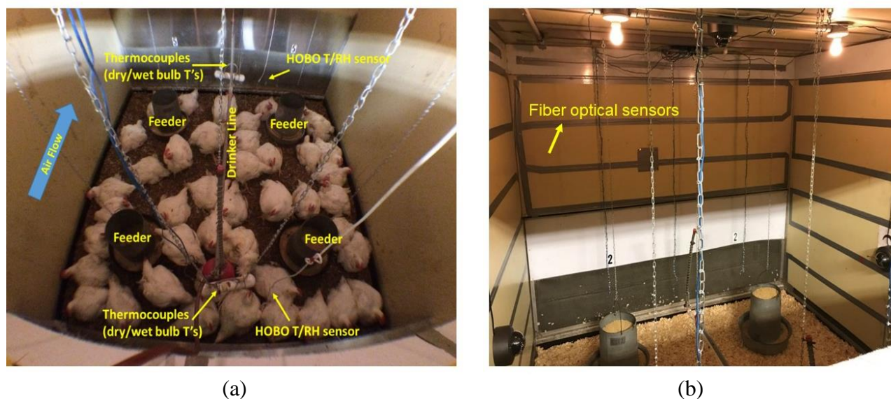
Figure 1. Locations of sensors, feeders, and drinker lines inside of the core chamber
