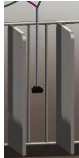
Figure 7. Design 3 CAD Drawing. Three-dimensional drawing of design option 3 with individual spray modules as opposed to a complete spray bar with nozzles for four stalls.
