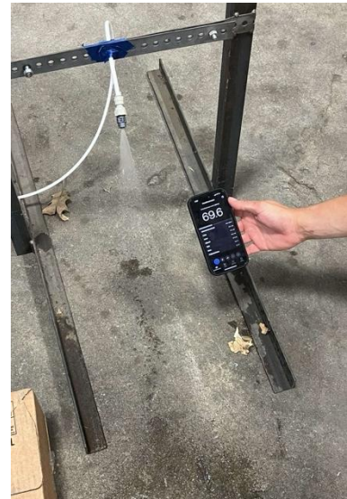
Figure 22. Noise Testing. Snapshot of sound assessment using the NIOSH app.
