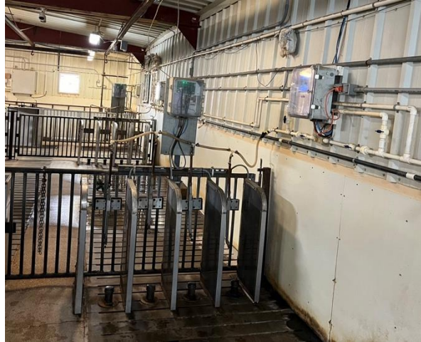
Figure 1. Swine Monitoring System Barn Configuration. Swine Monitoring System set up in the pig barn on the drinking stalls. Electrical box to the left on the wall shows a digital monitor of the weight system.
