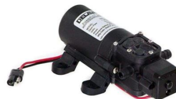
Figure 9. Selected Fluid Pump. Chosen fluid pump for the final design. Commonly used in small agricultural spray applications requiring low flow rates. The maximum flow rate is 1 gallon per minute, maximum output pressure is 40 psi, and power needed is 12 V. It also features self-priming and a 3/8" hose outlet barb.
