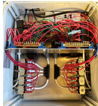
Figure 11. Polycarbonate Box Components. The top panel, located above the fluid assembly, plays a vital protective role, particularly when upright, guarding against potential leaks. The white rectangle represents the power source, supplying energy to the ARDUINO, relay switches, and solenoids via the terminal bars at the base of the electronic panel. Relay switches, depicted as small black boxes at the far ends of the panel, oversee critical functions. Situated centrally beneath the wires, the ARDUINO and voltage regulator circuit board optimize operational efficiency.
