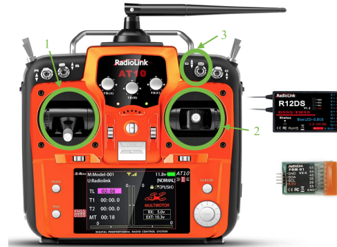
Figure 20. Image of the Radiolink AT-10 remote control. Label 1 is the joystick used for the drive wheels. Label 2 is the Joystick used for the ELAs. Label 3 is the switch for controlling the grippers.
