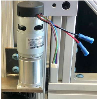
Figure 16. Selected motor to drive arms of gripping mechanism. 24 DC gear motor. Rated to supply 2.2 ft-lbs of torque. Mounted on the gripping mechanism as seen in photo.
