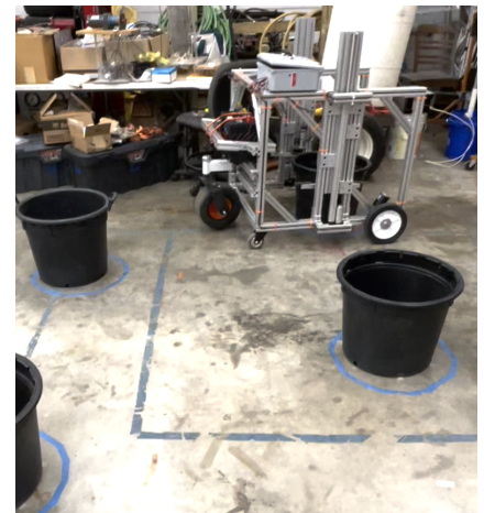
Figure 23-25. Pictures of PIPER navigating through the PNP staggered spacing. Fig. 23 on the left depicts PIPER being driven down the row. Fig. 24 in the middle shows the approach to a pot. Lastly, Fig. 25 shows PIPER surrounding a pot ready to grip and lift.
