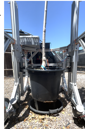
Figure 27. PIPER successfully gripping and lifting a 15-gallon potted maple tree in UT Nursery Complex.
