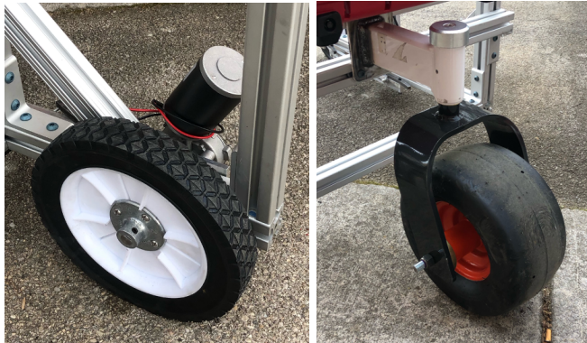
Figure. 8 & 9. To the left is a photo of the driven wheels. They have a 10 in diameter and are 1.75 in thick. To the right is the caster wheel that sits in the back of the chassis. The wheel has an 11 in diameter and is 6 in thick. The setup of the driven wheels and caster wheels allows the robot to drive similar to a forklift.
