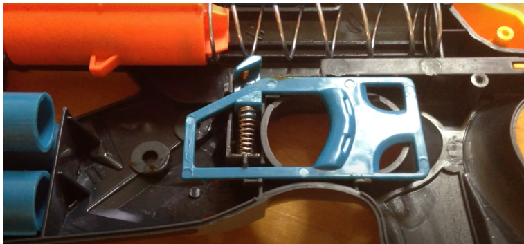
Figure 6: An example of the trigger mechanism planned to be used for the feed shut off
