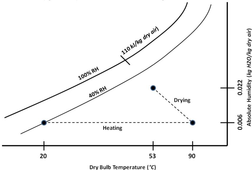
Initial moisture mass flow rate (kg H<sub>2</sub>O/min) in beets entering dryer =  $F_{x_f} = 25$  kg beets/min  $\times 0.87$  kg H<sub>2</sub>O/kg beets = 21.75 kg H<sub>2</sub>O/min
