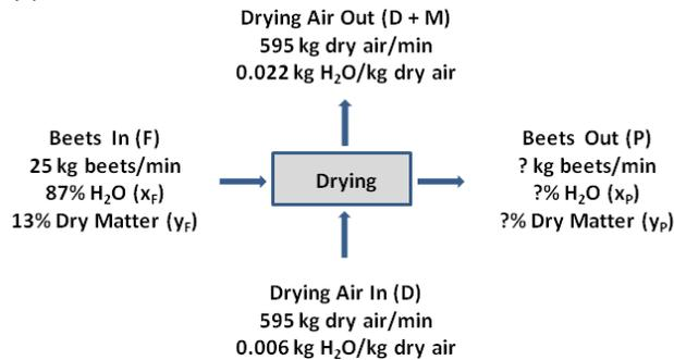
Moisture gain (kg H<sub>2</sub>O/kg dry air) by drying air =  $0.022 - 0.006 = 0.016$  kg H<sub>2</sub>O/kg dry air
