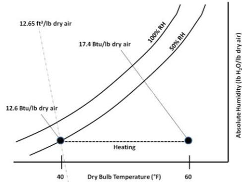
$$V_{\text{air in}} = 12.65 \text{ ft}^3/\text{lb}_{\text{da}}$$
